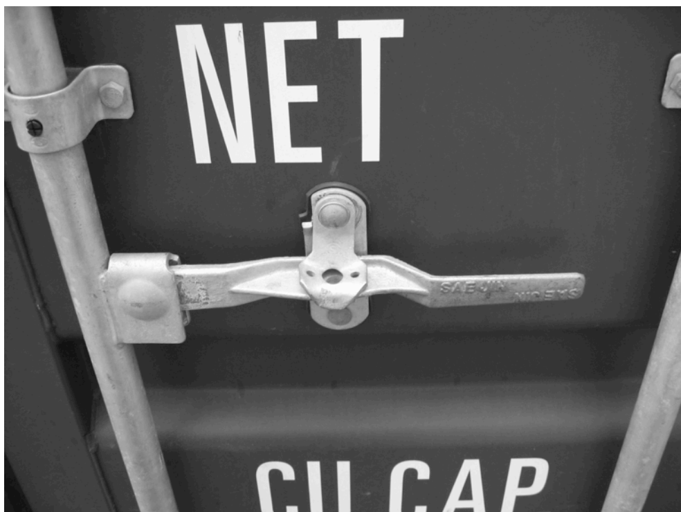
Figure 37: Container door handle (Source: Photo author's own)
