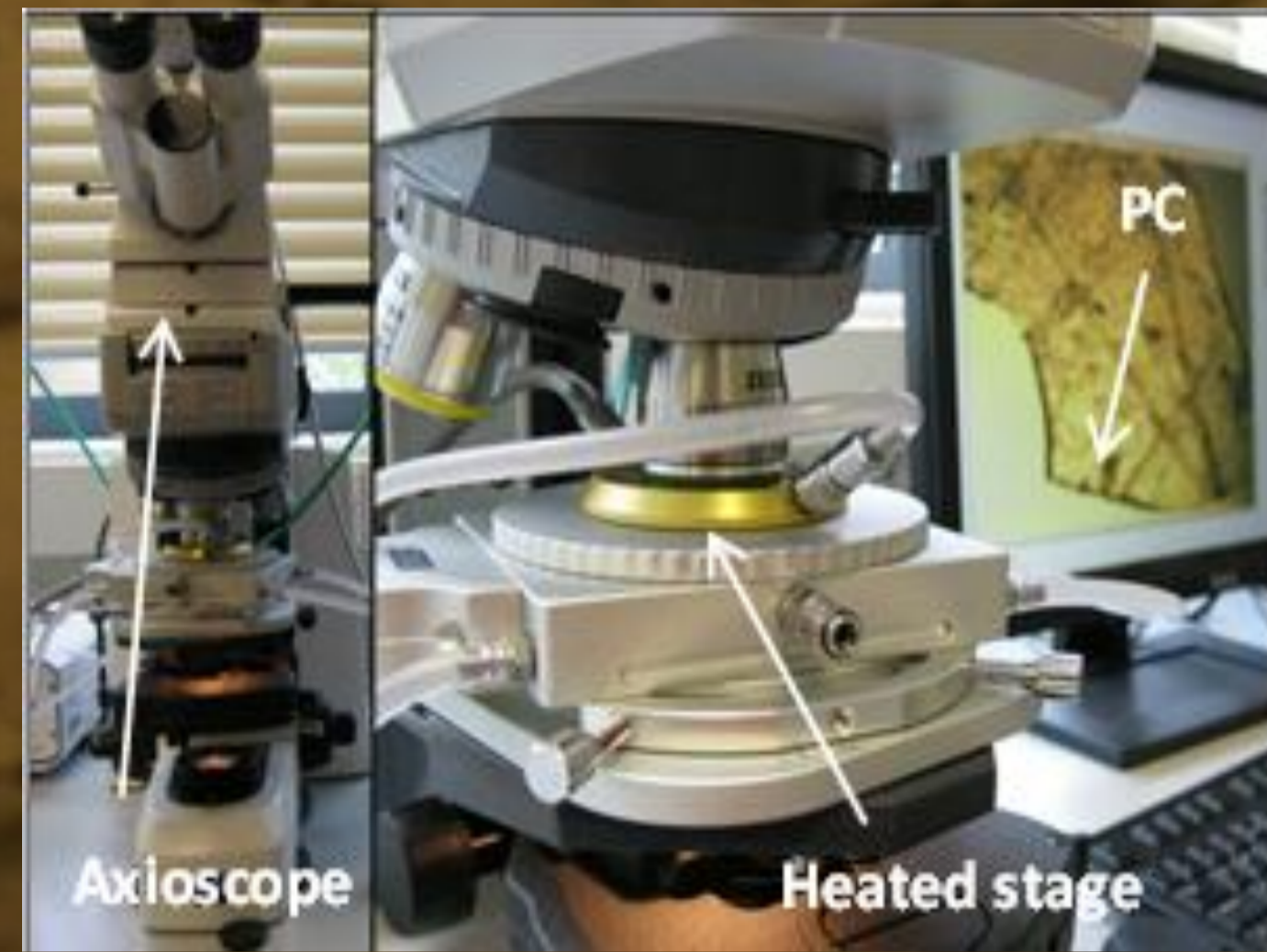
Fig 2. Hot-stage microscope setup 3 . Sample is placed inside a ceramic furnace (Linkam TS1500 heated stage), mounted on a Zeiss AxioScope.
