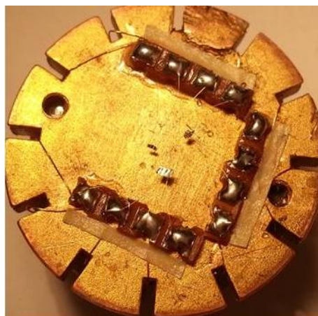
Figure 4.10: Resistivity puck with three samples mounted and connected with four gold wires using silver glue.
