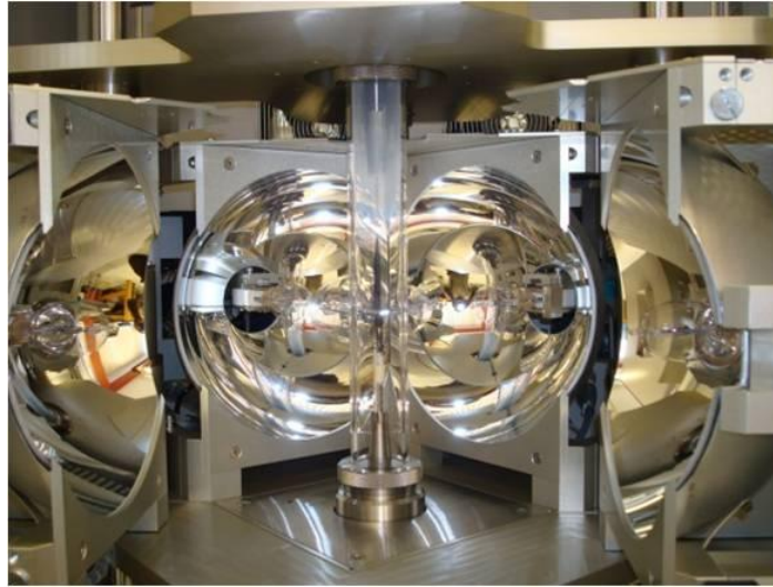
Figure 2.8: Optical floating zone furnace, with four Xenon lamps and the sample in the middle.
