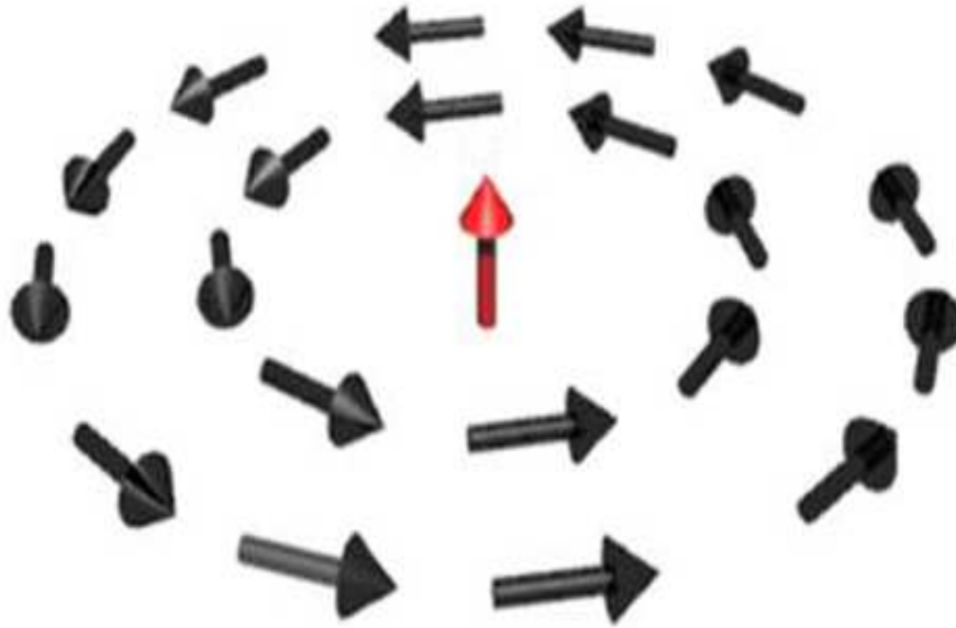
Figure 2.8: Illustration of the spin arrangement within a magnetic vortex [45].
