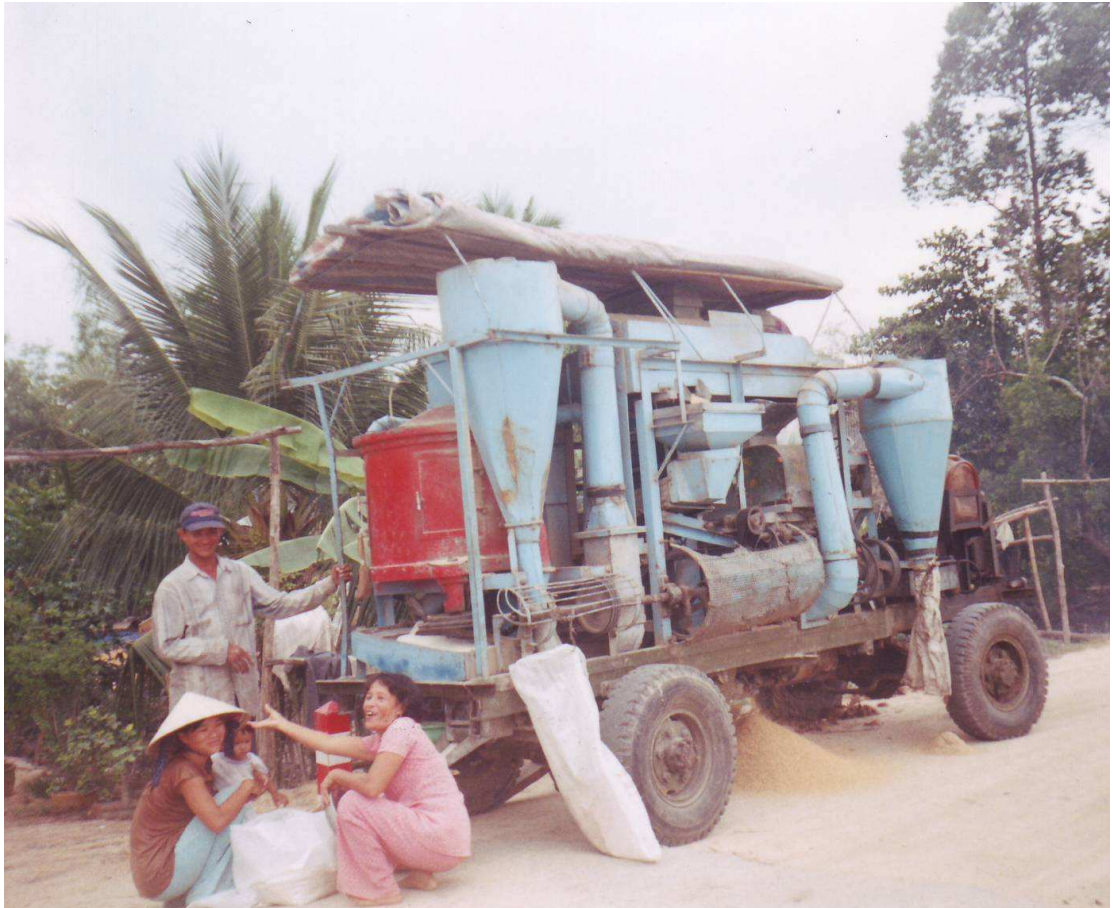
Figure 25 Travelling rice mill
